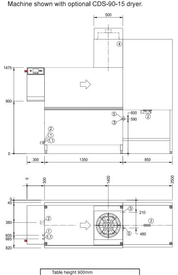
Machine height +/- 25mm feet adjustable
